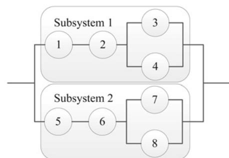
Fig. 4 Configuration of a hypothetical small series-parallel system
